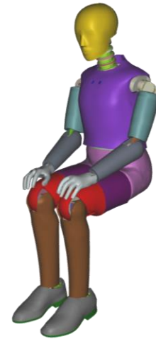
Figure 1: The ATD is based on the geometry of the Hybrid III 50 th percentile Male ATD.
