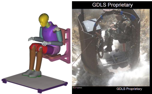
Figure 16: The ATD in the blast model at 100 msec. Left: Numerical model. Right: Image from high-speed video of Shot # 3. The seat and floor frame are displacement controlled with sampled values from the experiment.
