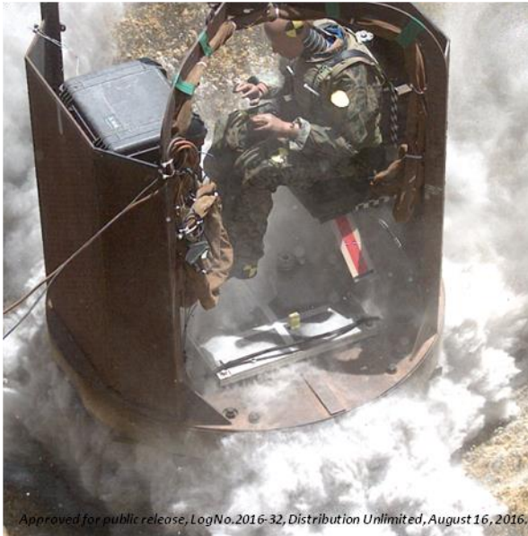
Figure 12: Blast experiments at General Dynamics Edgefield Test Site. Top: Initial position of the 90° test. Bottom: Motion of the fixture during the blast event.
